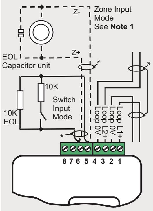
**S4 1-Output & 1-input module connection details**
