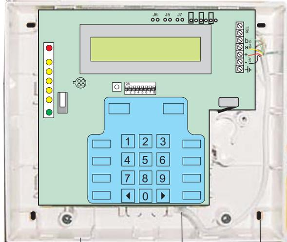
Thinned sections on sides of enclosure for cable entry
