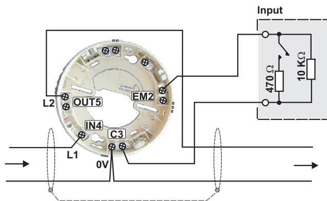
The input can accept signals such as fire, non fire or fault, these are configured during commissioning. As a fire input it is possible to connect a conventional Manual Call Point (non UK application only) with a series resistor of value 470 Ohms coupled with an end-of-line 10Kohms resistor. In this case the fire input is fully monitored for open or short circuit faults.
