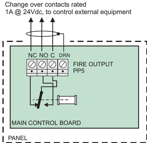
The relay is normally de-energised and operates with a fire event.
