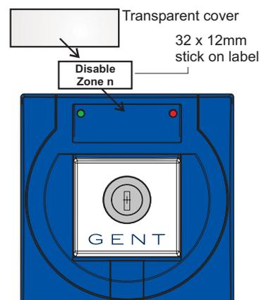
It is suggested that an A4 sheet white paper label 32 x 12mm is used, such as the one from RS, part number RS495 385. The required text can be printed onto the label. The label is stuck centrally inside the aperture behind the transparent cover. Ensure LEDs remain visible and are not covered by the label.
