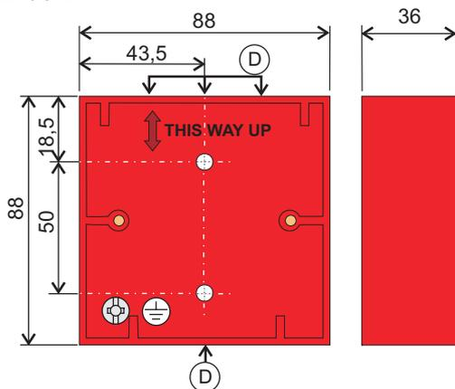
The back box has recessed centres 'D', 3 at the top and 1- at the bottom, a maximum of 2 are usable.
