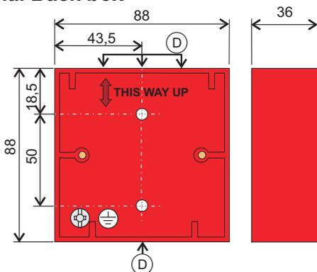
The optional back box has recessed centres 'D', 3 at the top and 1 at the bottom, a maximum of 2 are usable.
