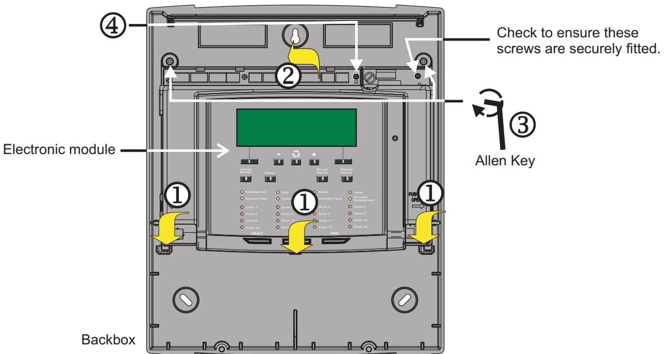
Locate the three tabs of the electronic module ① into the backbox and close the upper part ② of the module into the backbox and then secure the assembly by tightening the two captive screws ③ using the allen key. Ensure the two PCB fixing-screws ④ that provides earth bonding are securely fitted and are not loose.
