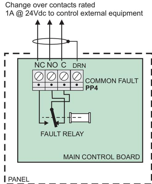
**i** The fault relay is shown in its normal state with panel powered up and with no active fault.
