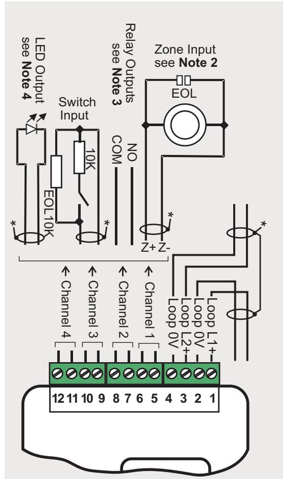
Note 1 - When the input is configured as a Zone input it is possible to attach conventional detectors and MCPs (with 470 Ohms or 3V9 zener diode in series with normally open contacts), maximum load is 2mA @ 24V nominal (18V minimum) with End-of-line capacitor.
