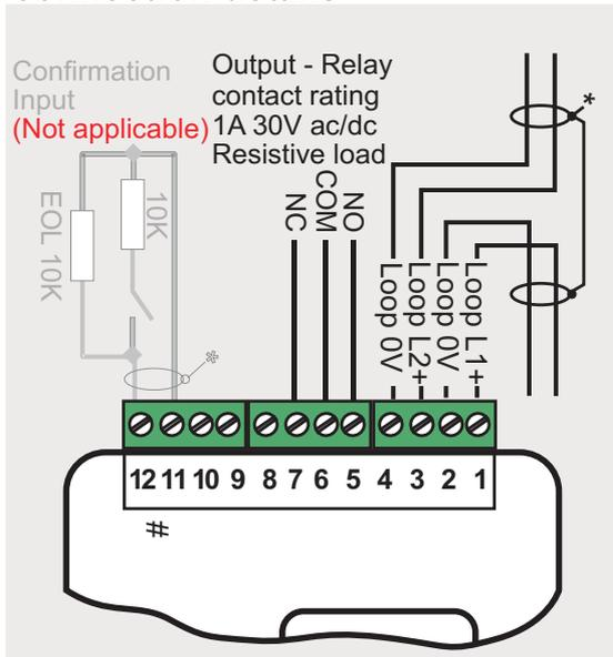
**S4 4-Input/Output module connection details**
