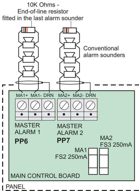
If master alarms are not being used then connect the 10K ohms End-of-line resistors to the master alarm terminals.
